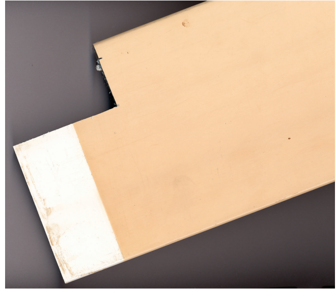
Discoloration: a real life example of a fence in a hot dry climate.
